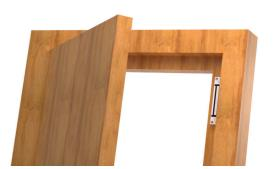
Those of the **shearlock** type are suitable for back and forth doors, both single and double-leaf (provided that one of them is fixed). The retention force we achieve is a shear force, as opposed to that with everyday electromagnetic locks, which is a tensile force.
