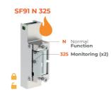
The DST (Dorcas Sliding Technology) system ensures mechanical opening, both in normal type strikes and reversed strikes, with preload of up to 20 kg. To provide additional security, the strike is equipped with a secondary system that ensures locking if opening is not electrically authorised.
