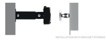
The magnetic door holder must be **mounted on the floor**, the counterplate is installed in the door leaf (placing it at least 150 mm away from the door's top or bottom closing edge). All parts must always be installed. Another option is to place a wall magnetic door holder with bracket RT/SR220 fixed to the floor.
